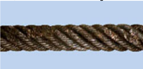
Heat, Chemical or Electrical damage
