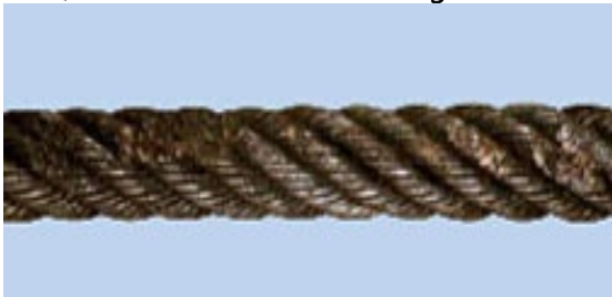
Heat, Chemical or Electrical damage
