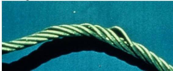
**Heat, Chemical or Electrical damage**
