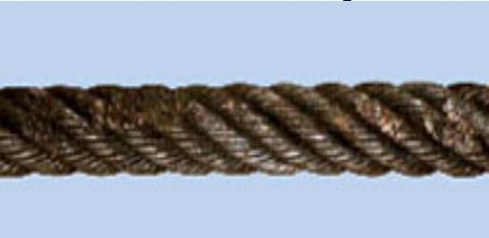
**Heat, Chemical or Electrical damage**
