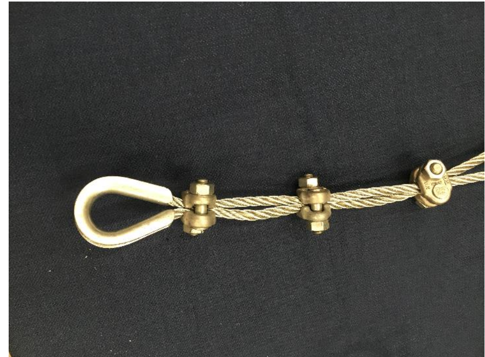
Fist grips - 3 improperly torqued (10 ft-lbs)
