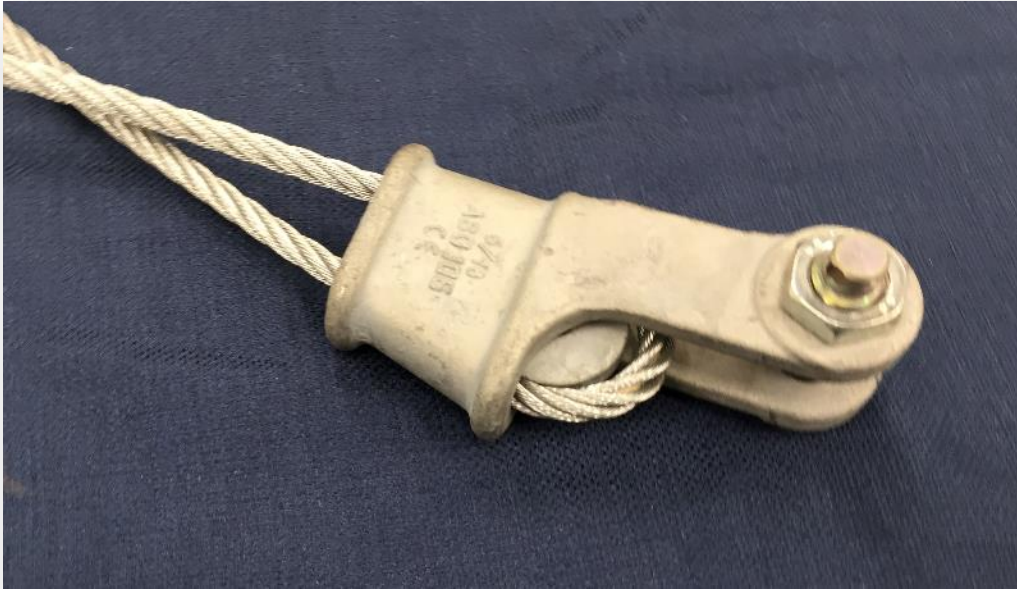
5/16” wedge socket (correctly sized for wire diameter)
