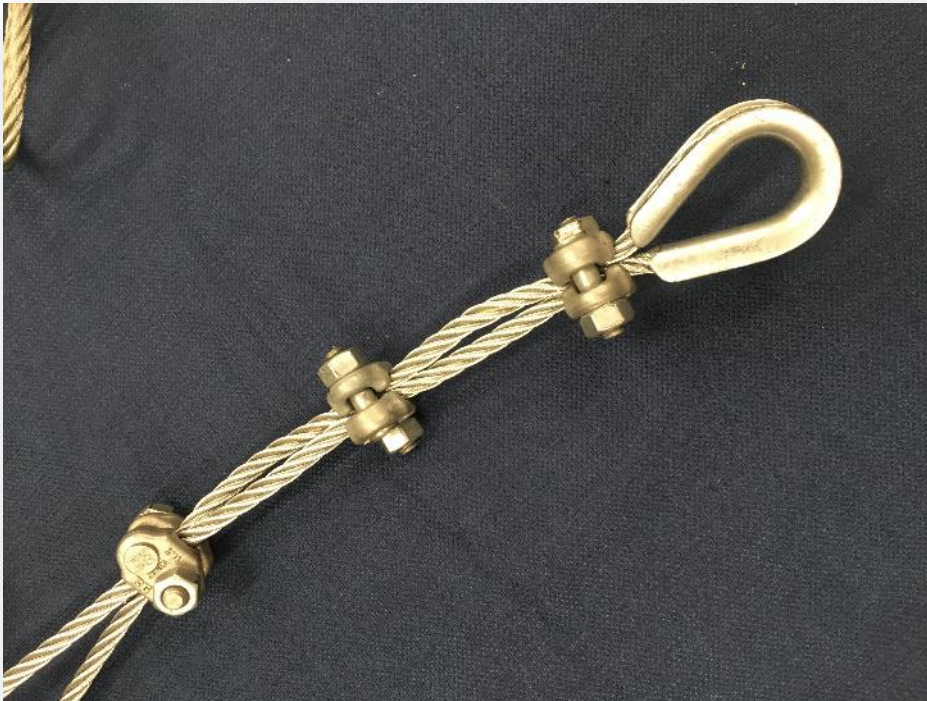
Fist grips - 3 properly torqued (30 ft-lbs)
