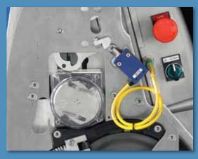
LNX has an internal over-speed device that will automatically reset by going in the upward direction.
