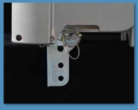
Fold-up stirrup strap design enables hoist to be maintained and stored easily.
