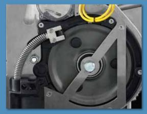
Solid sheave traction mechanism grips wire rope for ascent and descent using innovative roller system.
