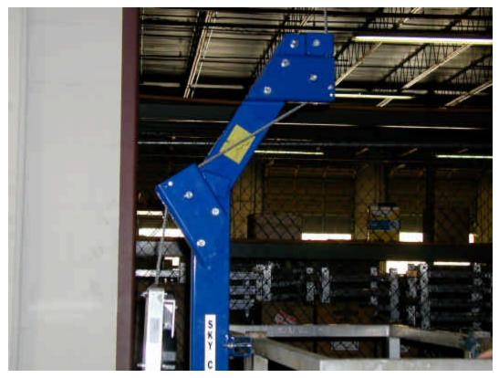
Figure 6 - Close-up view showing routing of wire rope through stirrup and into hoist. Path of wire rope is through top of stirrup, under top pulley, over bottom pulley, through sky lock, and into hoist.
