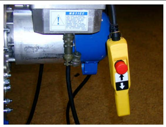
Figure 11 - View of an optional 6-Foot Pendant Control (P/N: 41021752-6) and its connection on the Compact hoist. Pendant Control is connected by simply removing the Jumper Plug connection from back of hoist and connecting the Pendant Control connection\*. Hoist can then be operated by either the hoist mounted controls or the pendant controls.
