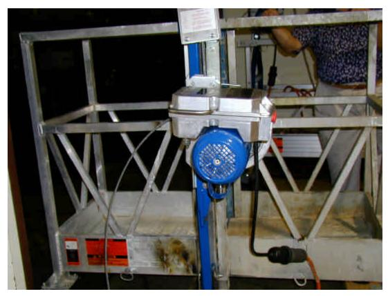
Figure 1 - Side view of Compact hoist mounted on Walk-Thru stirrup of MKD Work Cage.
