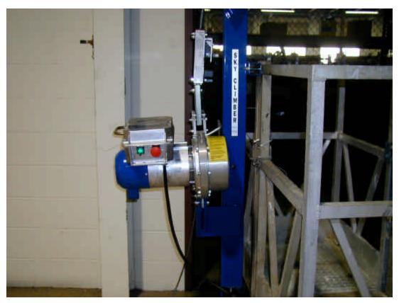
Figure 3 - Front view of Compact hoist mounted on Walk-Thru stirrup of MKD Work Cage.
