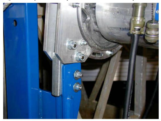
Figure 8 - Close-up of hoist's stirrup strap mounted on Walk-Thru stirrup of MKD Work Cage.
