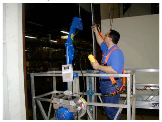
Figure 10 - Operator using the optional pendant controls of Compact hoist mounted on Walk-Thru stirrup of MKD Work Cage.
