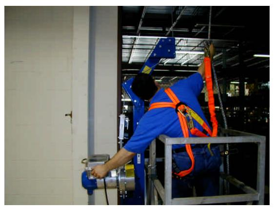
Figure 9 - Operator using the hoist controls of Compact hoist mounted on Walk-Thru stirrup of MKD Work Cage.
