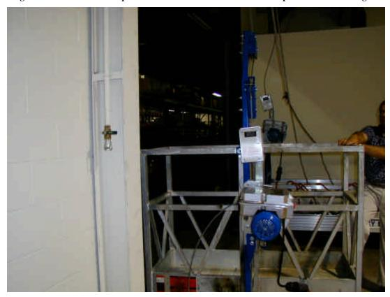
Figure 2 - Complete side view of Compact hoist mounted on Walk-Thru stirrup of MKD Work Cage.
