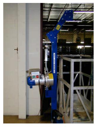
Figure 5 - Complete front view of Compact hoist mounted on Walk-Thru stirrup of MKD Work Cage. Shows routing of wire rope through stirrup and into hoist.
