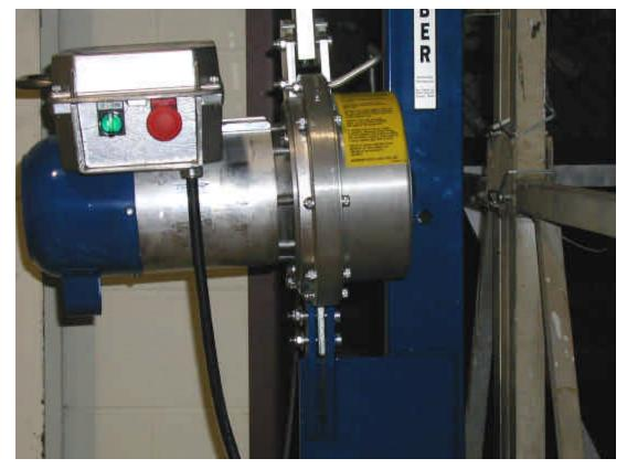
Figure 4 - Close-up front view of Compact hoist mounted on Walk-Thru stirrup of MKD Work Cage.
