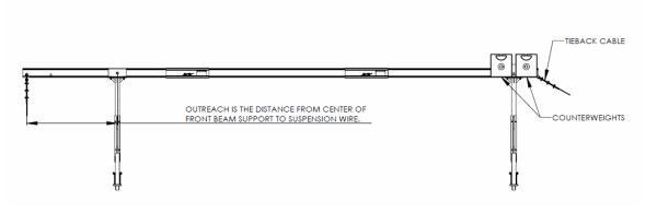
NO. OF 50LB COUNTERWEIGHTS REQUIRED PER BEAM ASSEMBLY
