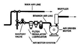
Check the direction of the motor airflow. A single rotation motor will operate properly only in one direction. Single rotation motors require a sound absorber to be connected to the air port. Remove the plastic shipping plugs from the ports. Save plugs for future use during shutdown.
